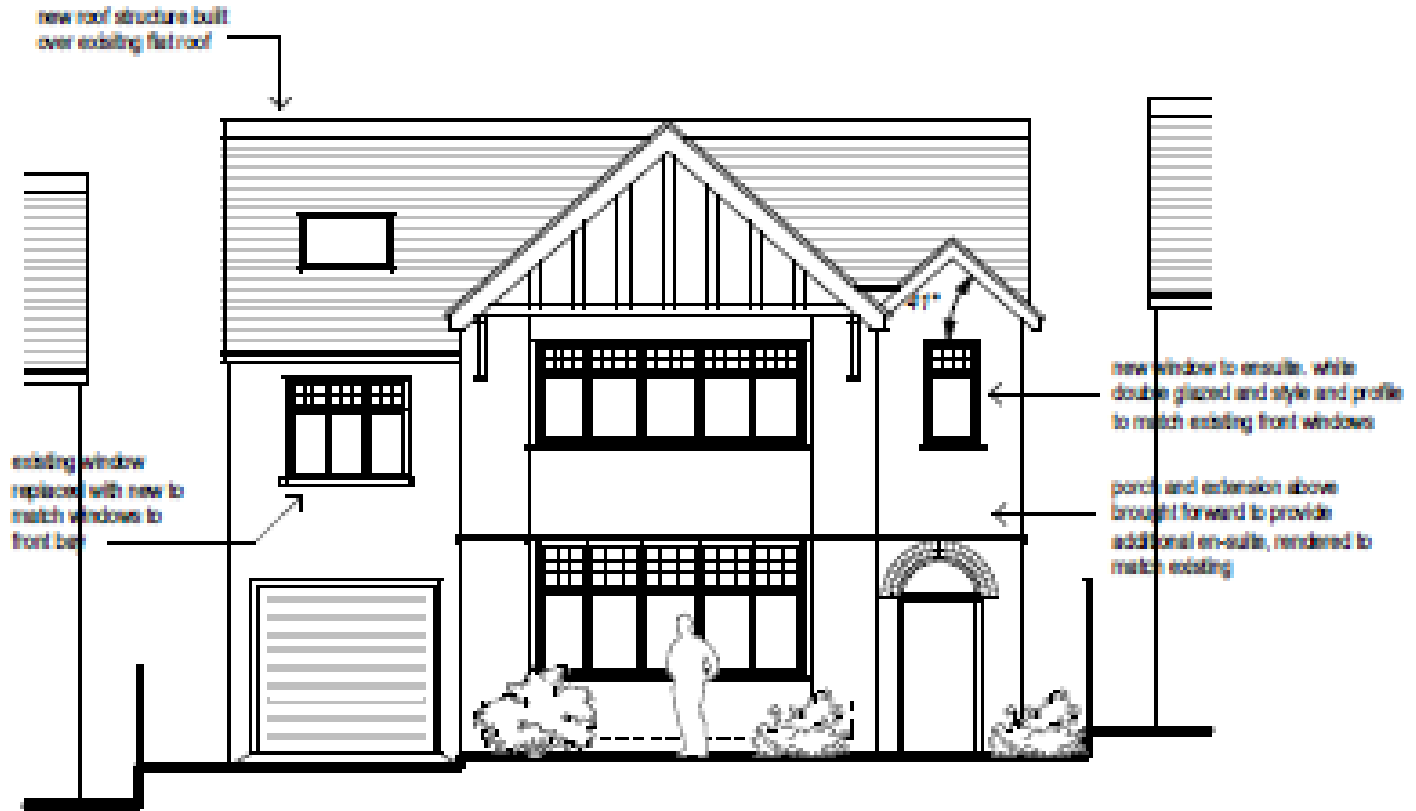
SOUTH WEST ELEVATION
